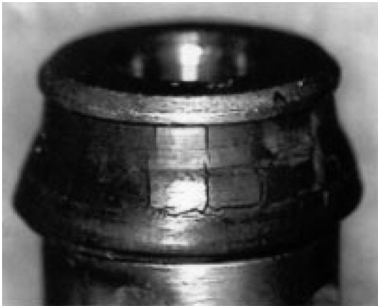
Photo 2 Cracking of check valve seal
